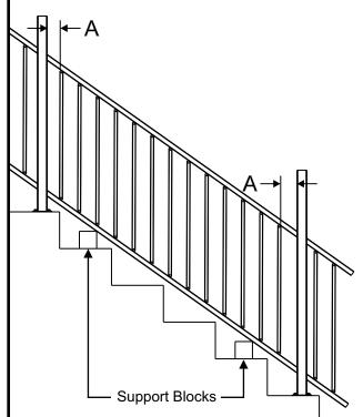
Use Fe<sup>26</sup> Adjustable Panel to determine the angle of stair installation. To do this use support blocks resting on the stair tread. Position support blocks so that the position of the bottom rail meets the spacing requirement of your building code.
